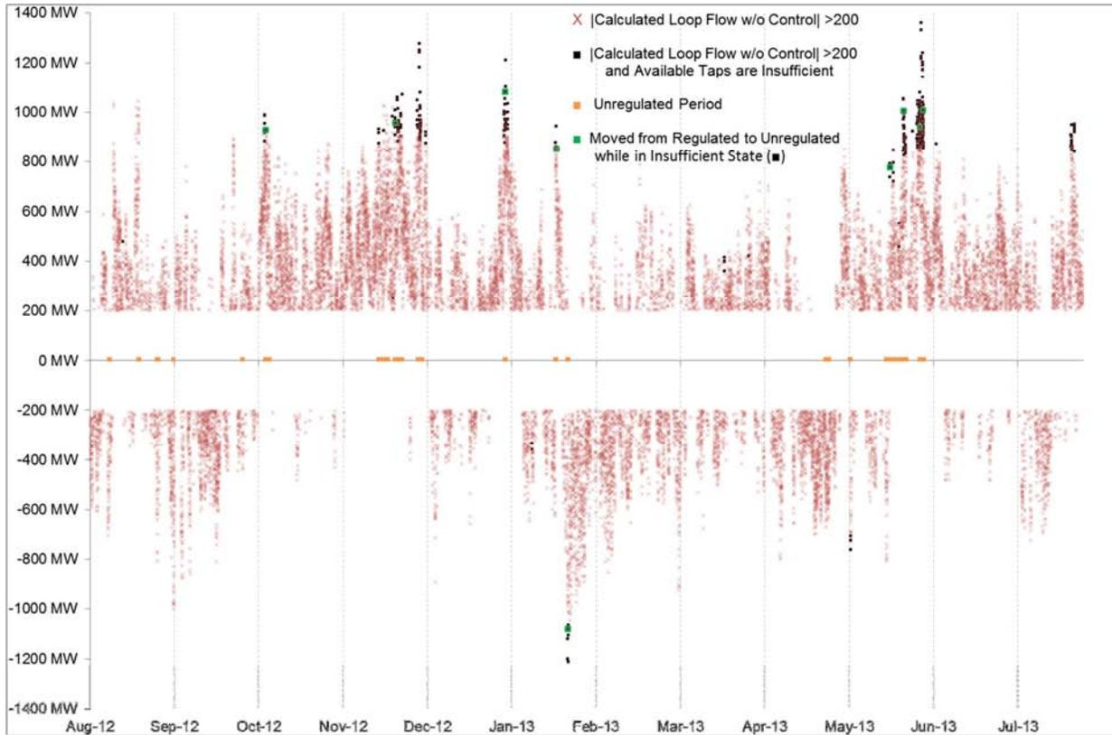
Figure 15 - Calculated Loop Flow without PAR Control Outside +/-200MW, 8/1/2012-7/31/2013
